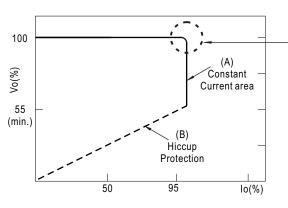
Typical LED power supply I-V curve
